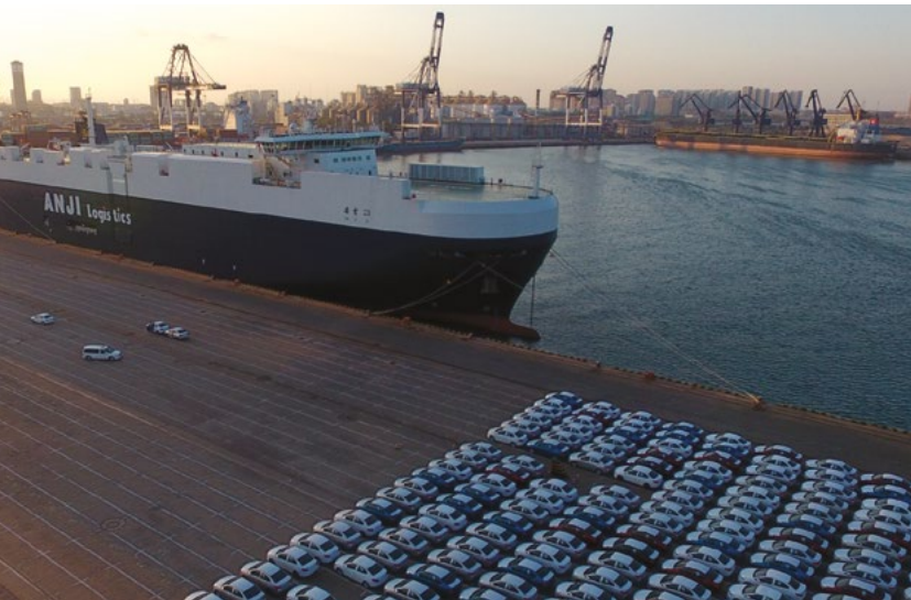
Picture: ANJI 23 , 10 decks incl. 2 hoistable. 56,794 square meters equivalent to 3,800 CEU. Delivered in April 2017 by CSC Jinling Shipyard in China to and operated by Shanghai Ansheng Automotive Shipping.
