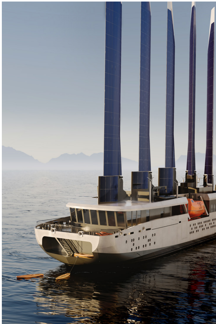
Figure 7: 70m cruise-expedition vessel CAPTAIN ARCTIC with the world's first solar-powered wing rig. Credit: Bureau Veritas.
