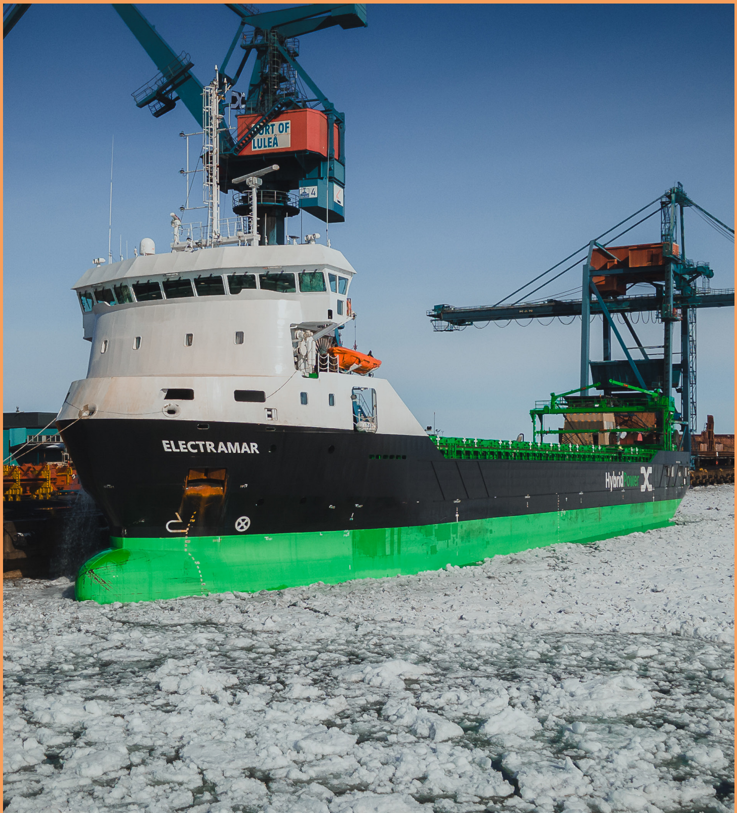
ELECTRAMAR Ice class 1A general cargo carrier with hybrid propulsion, 5,350 Dwt, built by Chowgule (India), ATOB@C (part of ESL Shipping Ltd.), December 2023. Copyright: AtoB@C Shipping
