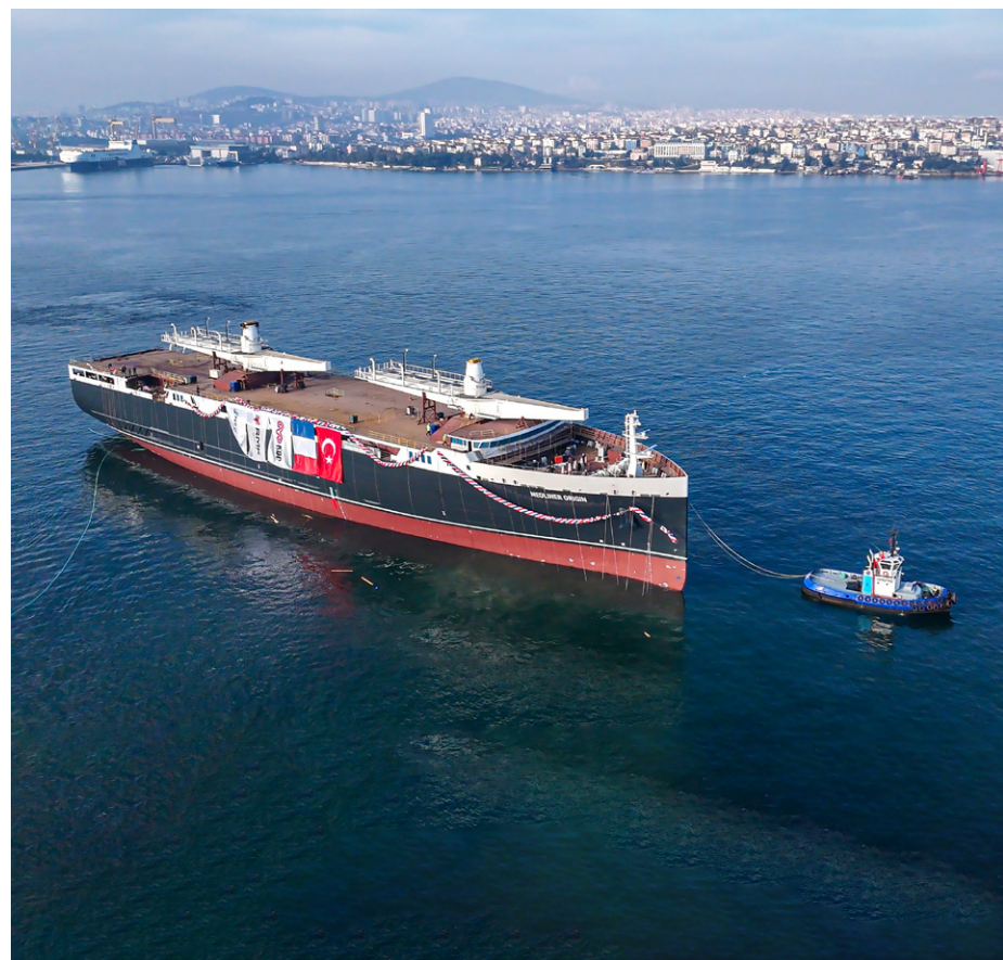
Figure 8: Ro-Ro vessel Neoliner Origin, will be fitted with two Solidsail rigs (designed by Chantiers de l'Atlantique), using wind as main propulsion, under construction in RMK Marine (Türkiye)
