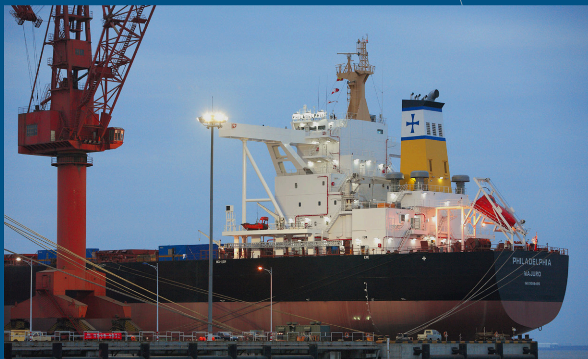
M/V PHILADELPHIA Newcastlemax Bulk Carrier, 206,040 Dwt, built by Shanghai Jiangnan- Changxing Shipbuilding Co., Ltd., managed by Diana Shipping Services S.A., delivery year 2012.
