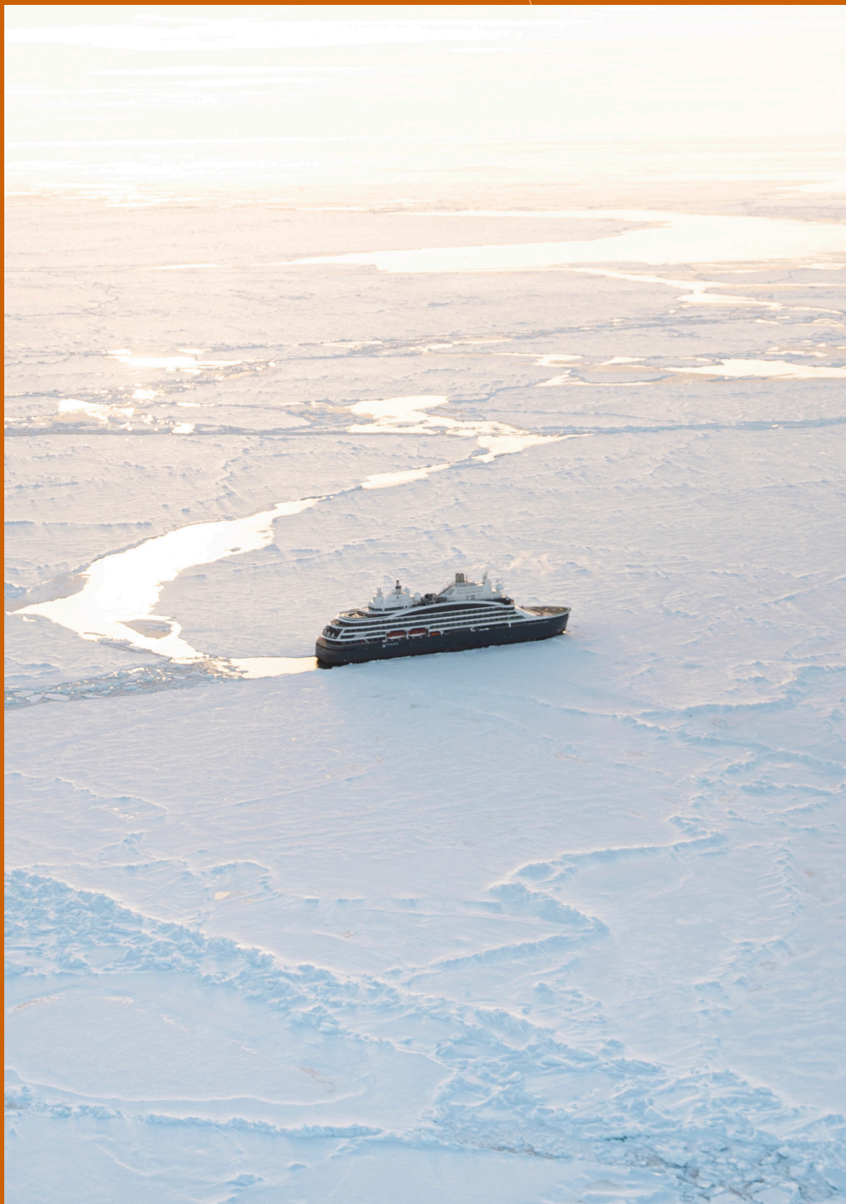
LE COMMANDANT CHARCOT Hybrid electric polar exploration vessel, 31,757 Gt, 150m in length, 28m beam, Polar Class 2 (PC2) icebreaker, built by VARD (Fincantieri). Hull constructed in Tulcea, Romania, and final outfitting in Søviknes, Norway, operated by PONANT, delivery year 2021.
