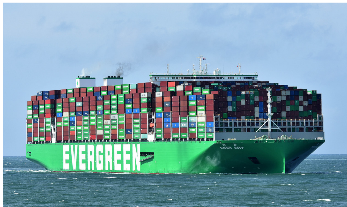
EVER ART Container vessel, 23,992 teu, built by Samsung H.I., operated by Evergreen, delivery year 2022. Copyright: C.H. Mercier
