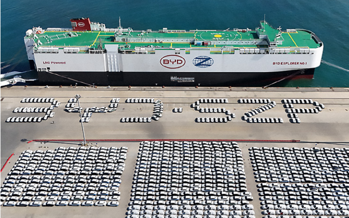
BYD EXPLORER NO. 1 Car carrier with post-Panamax beam and with approx. 59,000 sq m on 12 decks equivalent to approx. 7,000 CEU with 4 hoistable decks, endowed with dual-fuel LNG propulsion. Delivered in January 2024 by CIMC Raffles in China to Zodiac Maritime and operated by BYD.
