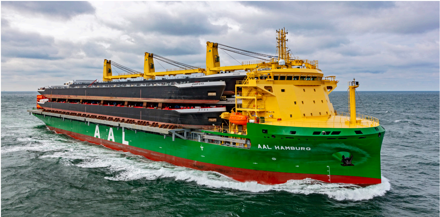
MV AAL HAMBURG - MPP / Super B-Class / 32,000 Dwt / built July 2024 at Guangzhou Wenchong / Owner/Operator: Austral Asia Line / Copyright: Austral Asia Line
