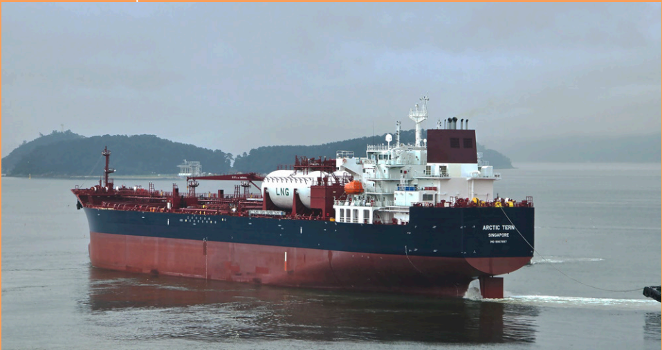
ARCTIC TERN MR2 Chemical/Oil Products Tanker of 49,037 Dwt, built by K Shipbuilding, South Korea, delivered 2024. The first Dual Fuel Diesel/LNG powered MR Tanker. Fully IMO 2 class with 20 tank segregations for optimal flexible cargo handling. On long-term charter to Louis Dreyfus Company (LDC).
