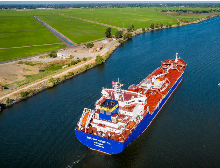
MT BOCHEM HOUSTON 25,000 Dwt stainless steel chemical tanker by China Merchants Jinling Shipyard (Yangzhou) Dingheng for CMB.TECH, delivered in June 2023
