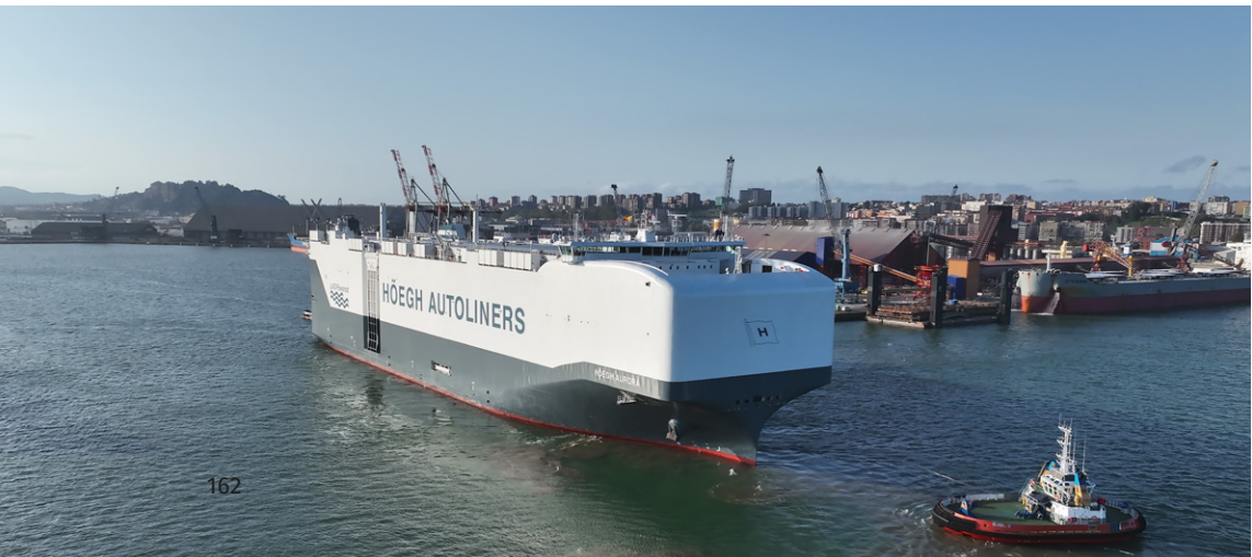
HØEGH AURORA First in the Aurora series of car carriers with post-Panamax beam and with approx. 75,000 sq m on 14 decks equivalent to approx. 9,100 CEU with 5 hoistable decks, endowed with multi-fuel propulsion. Delivered in August 2024 by CMHI Jiangsu in China for, and operated by, Høegh Autoliners.
