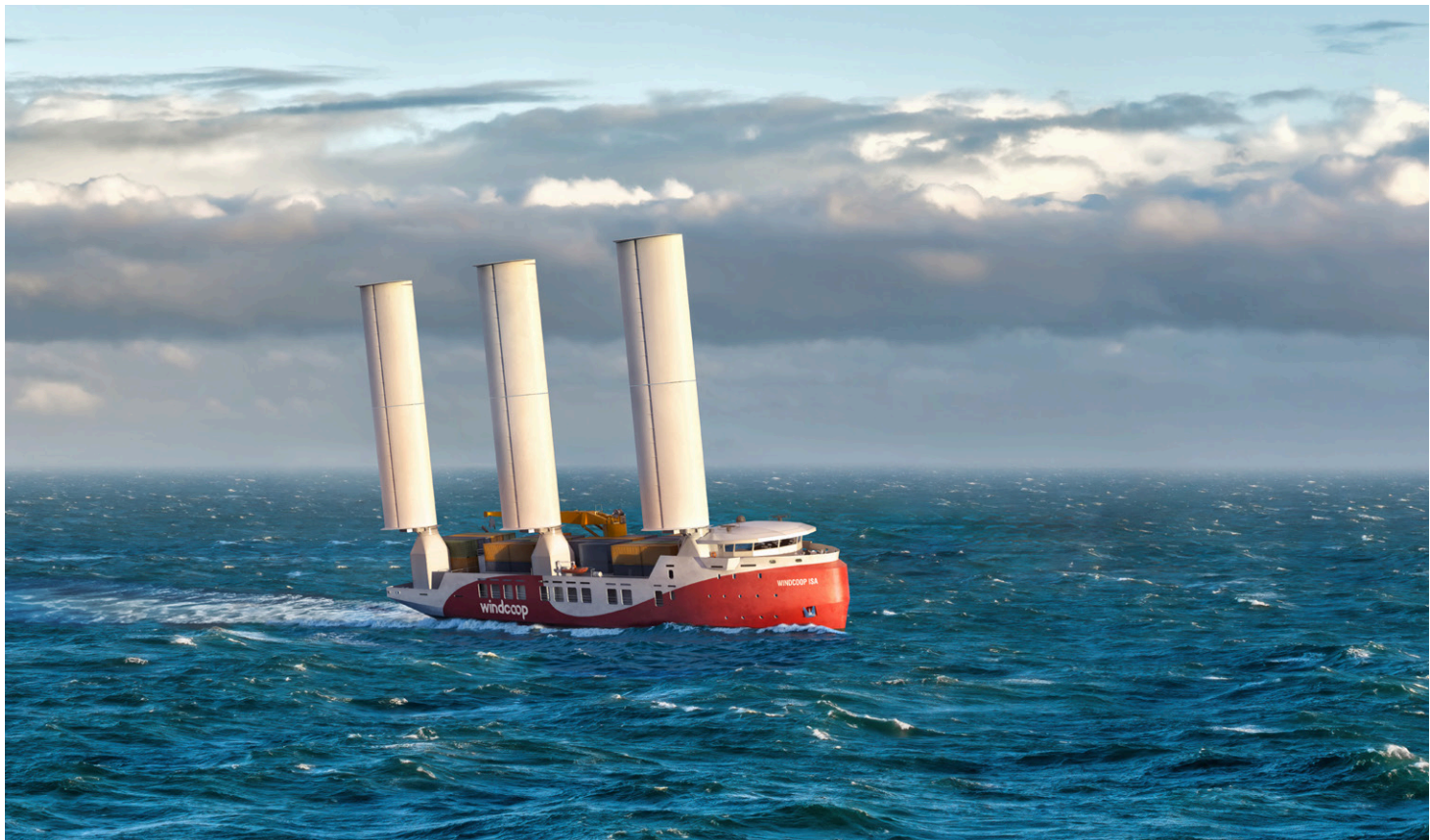
Figure 9: The 85m wind-powered cargo ship design by Windcoop for sustainable maritime transport. Copyright © 2025 Windcoop.
