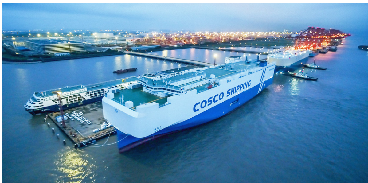
LIAO HE KOU Car carrier with post-Panamax beam and with approx. 59,000 sq m on 13 decks, equivalent to approx. 7,500 CEU with 4 hoistable decks endowed with dual-fuel LNG propulsion. Delivered in July 2024 by Xiamen Shipbuilding Industry in China to COSCO Shipping Specialized Carriers and operated by COSCO Shipping Car Carriers.
