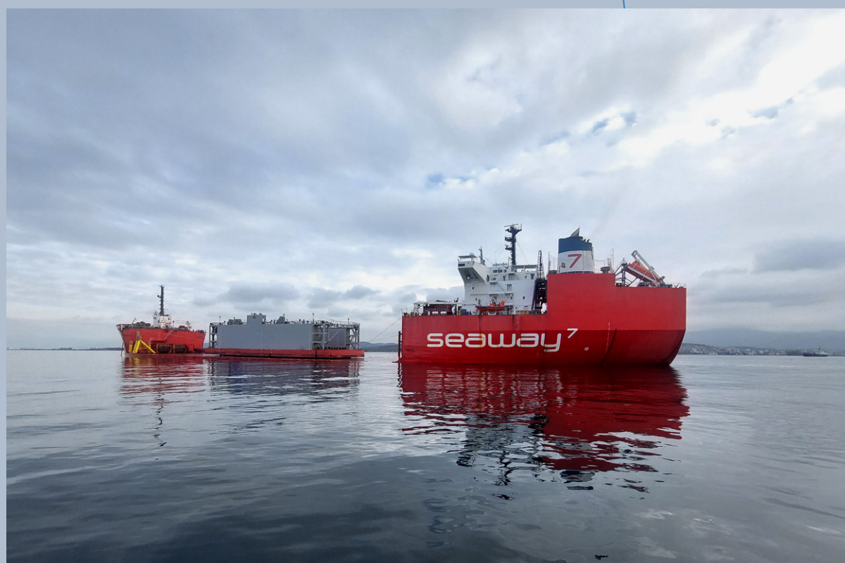
SEAWAY EAGLE, semisubmersible, converted from a tanker in 2006, Seaway7. Copyright : SEAWAY EAGLE
