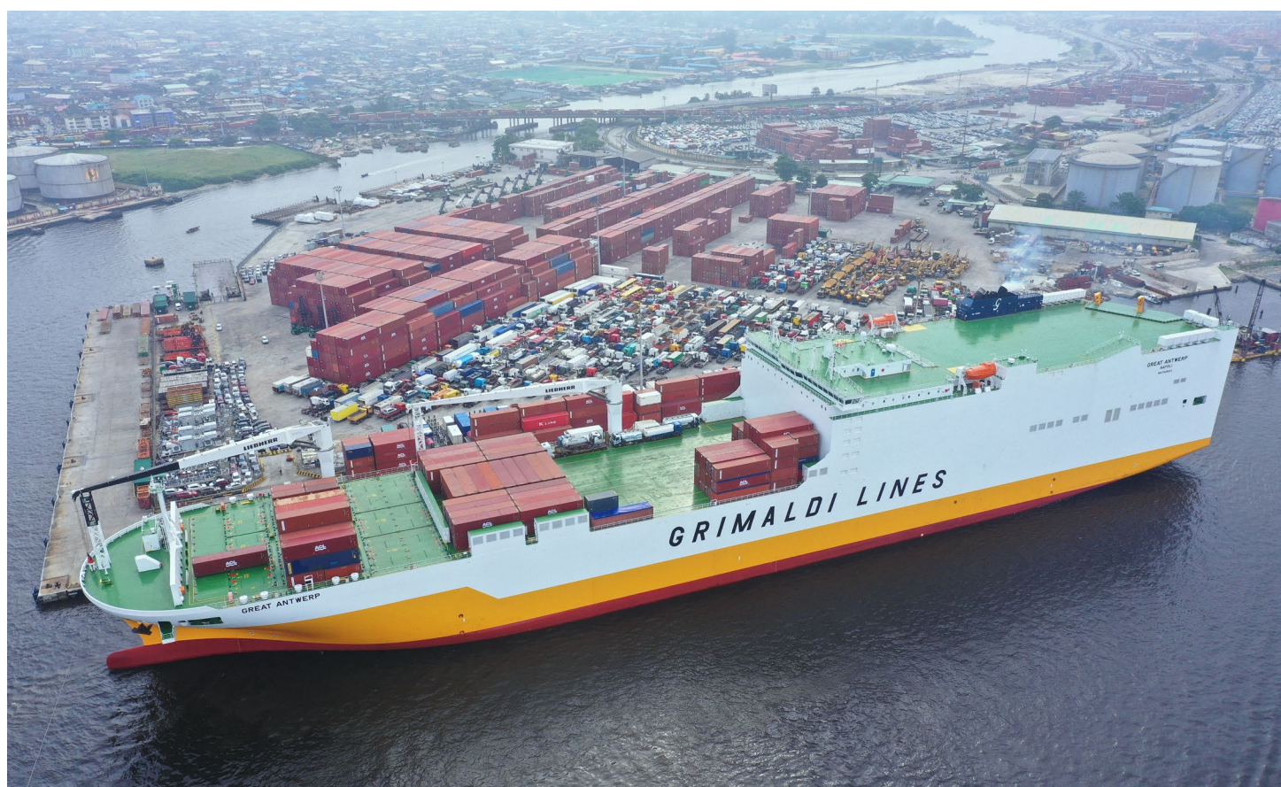
Image: GREAT ANTWERP, ConRo with 4700 LM + 2500 CEU + 2000 teu capacity. Delivered in April 2023 by Hyundai Mipo Dockyard in South Korea to and operated by Grimaldi.
