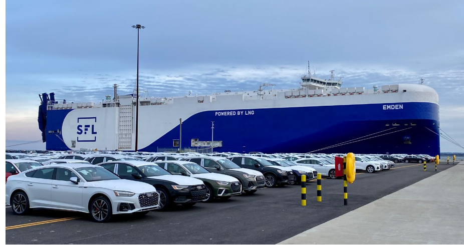
Image: EMDEN, car carrier with post-Panamax beam and with approximately 59,000 square meters on 12 decks equivalent to approximately 7,000 CEU with 4 hoistable decks endowed with dual-fuel LNG propulsion. Delivered in September 2023 by Guangzhou Shipyard International Co. Ltd. (GSI) in China to SFL Corporation Ltd. (SFL) and operated by Volkswagen Konzernlogistik (VWKL).
