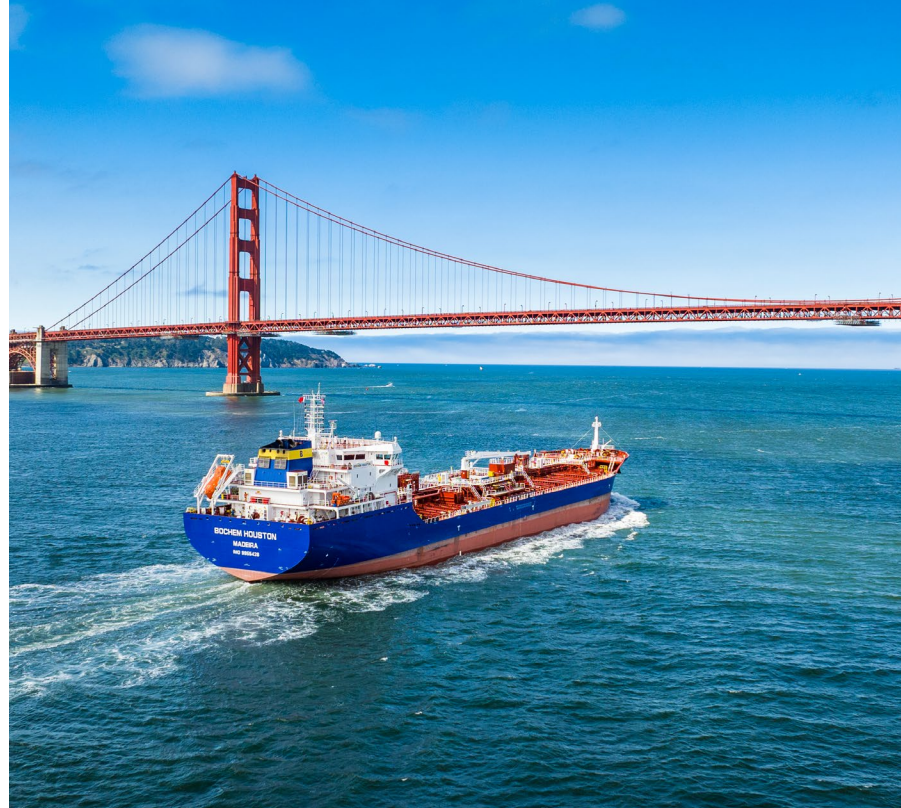
Image: MT BOCHEM HOUSTON, 25,000 Dwt stainless steel chemical tanker, built by China Merchants Jinling Shipyard (Yangzhou) Dingheng to CMB N.V., delivered in 26 June 2023.
