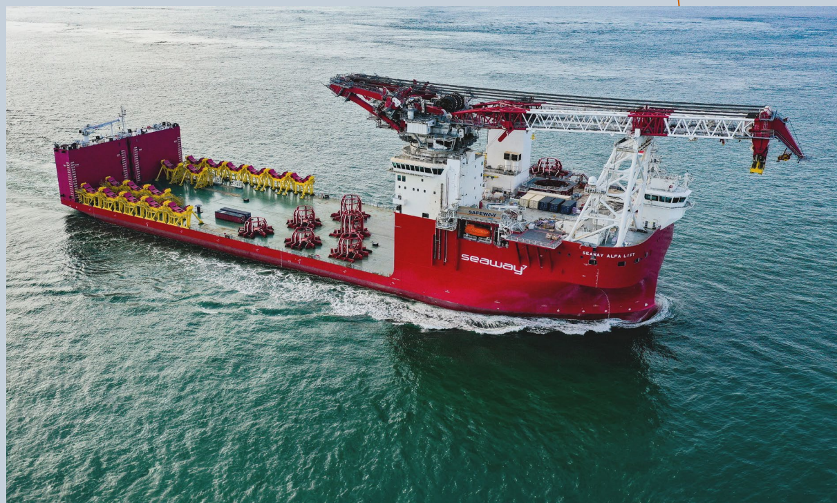
Image: SEAWAY ALFA LIFT, Foundation Installation Vessel, 8,000m 2 deck area and 3,000t crane capacity, built in 2023, Seaway7.
