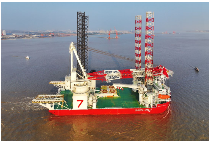
Image: SEAWAY VENTUS, Wind Turbine Installation Vessel, 4,600m 2 deck area and 2,500t crane capacity, built in 2023, Seaway7.
