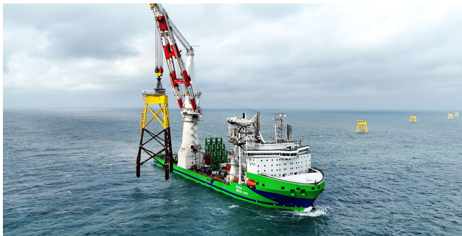
Image: GREEN JADE, Foundation Installation Vessel, 8,232m 2 deck area and 4,000t crane capacity, built in 2023, DEME. Copyright: DEME Group.
