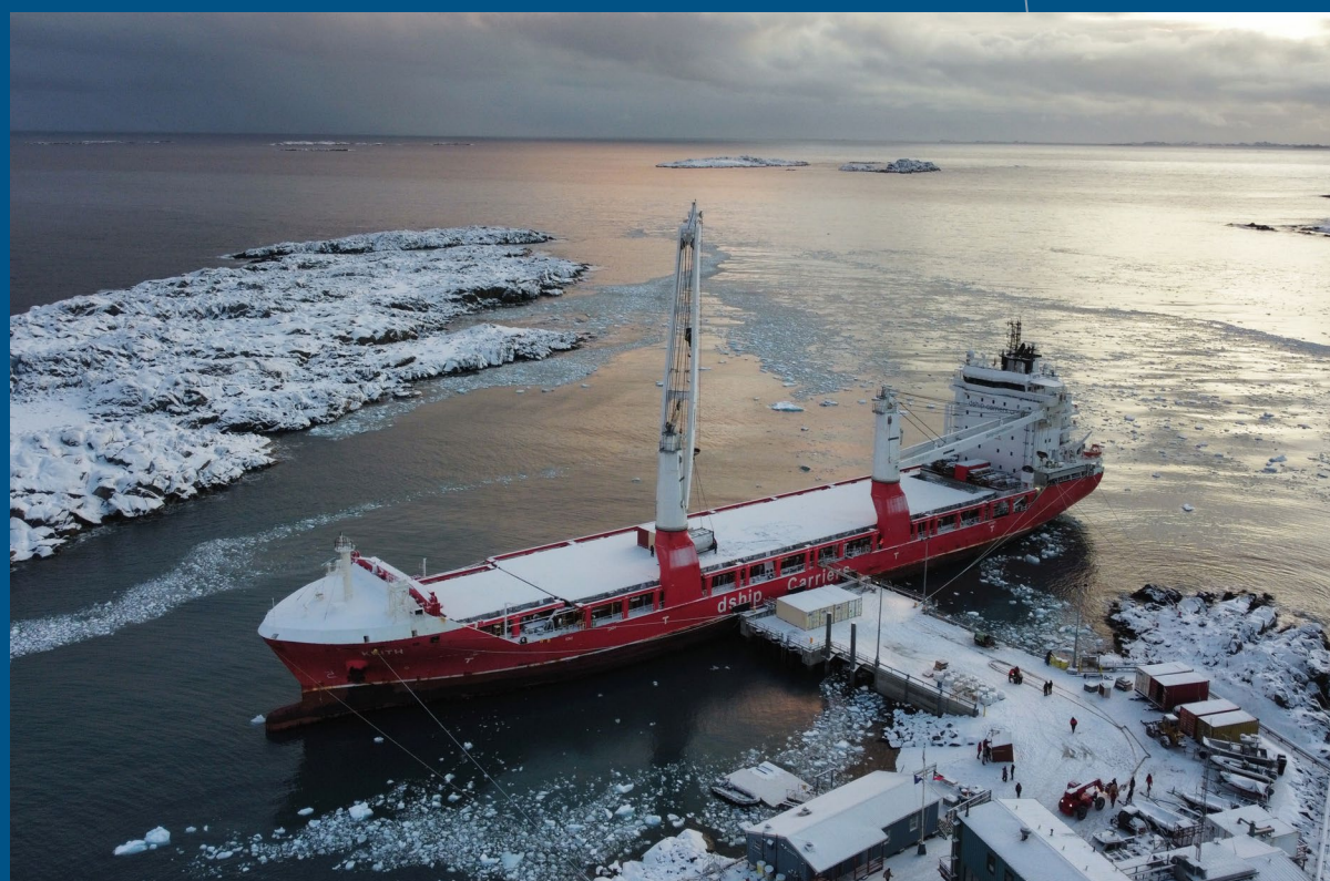
Image: MV KEITH — F500 design, built September 2019, 12,248 million Dwt on 8.10 m draft, gear 2x250 mts cranes combinable to 500 mts, operated by dship Carriers, shipyard: Taizhou Sanfu. Copyright: Dship Carriers.
