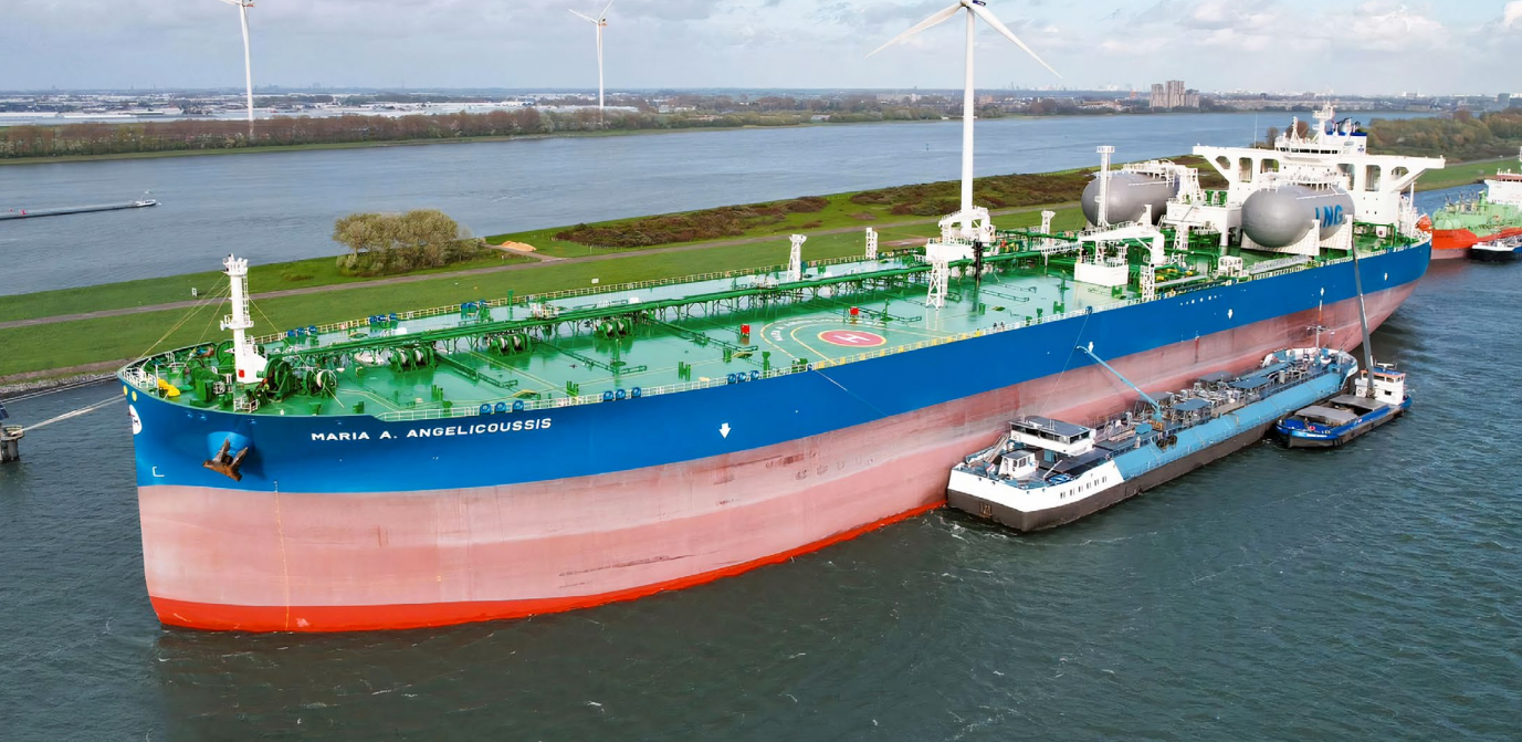
Image: Mt MARIA A. ANGELICOUSSIS — LNG dual-fuel VLCC, 320,917 mt Dwt built by Samsung Heavy Industries and operated by Maran Tankers, delivered in 2023.
