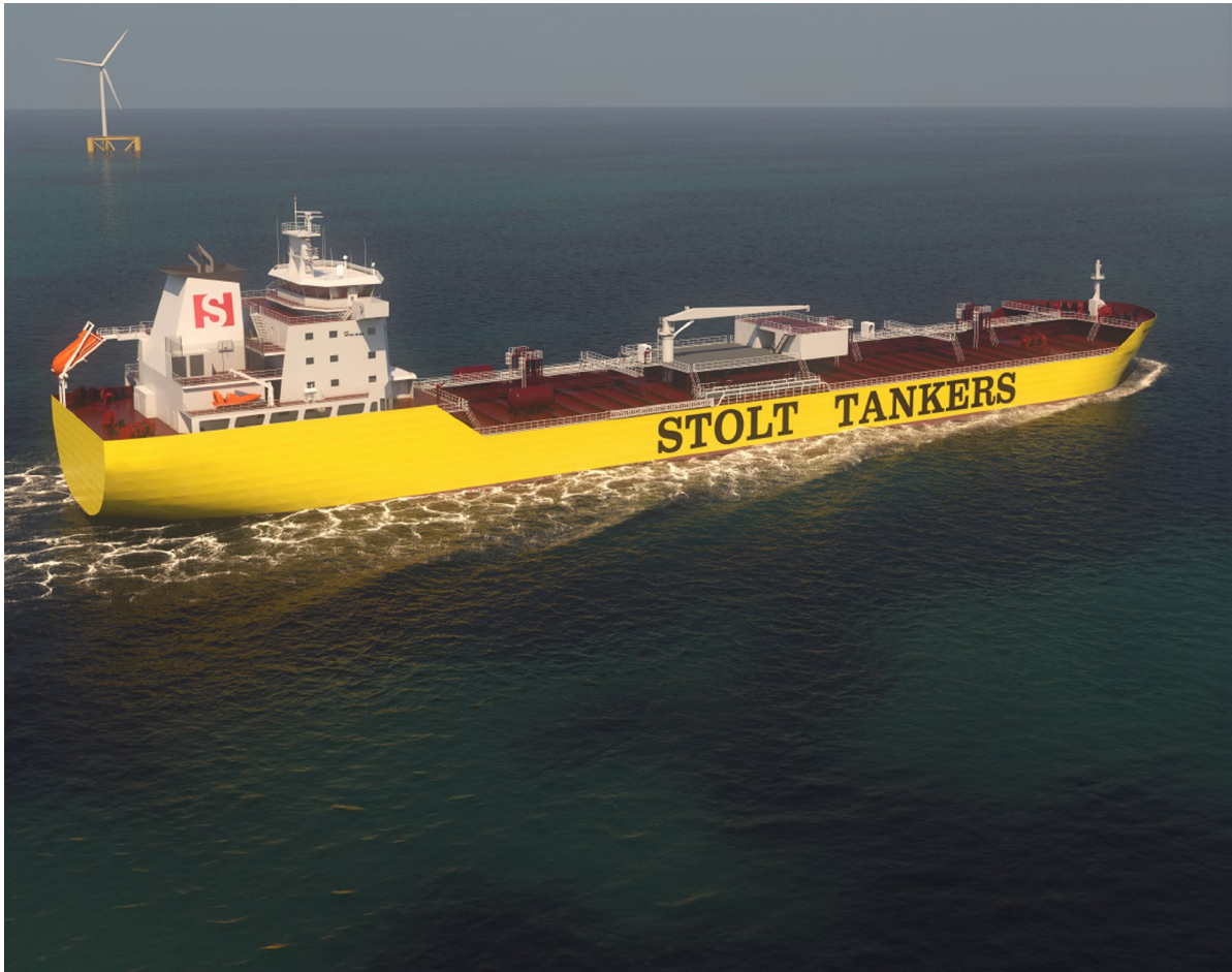
Image: Rendering of a 38,000 Dwt stainless steel chemical tanker, part of a large series, to be built for Stolt Tankers at Wuhu shipyard (China).
