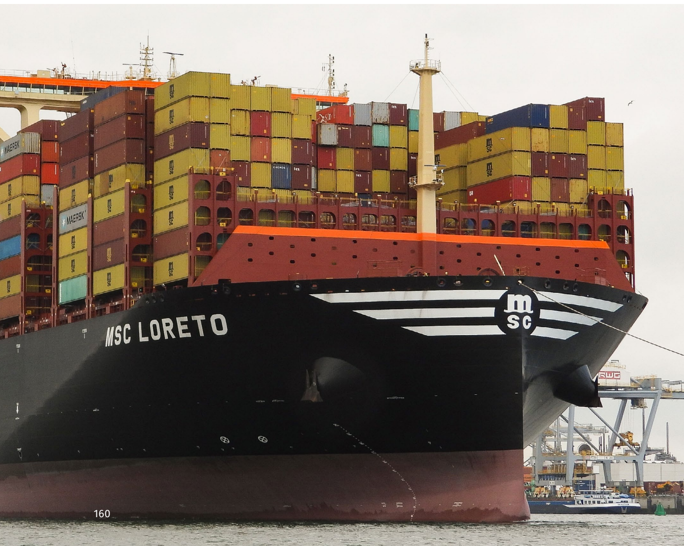
Image: The 24,346 teu MSC LORETO, delivered in April by Yangzijiang Shipbuilding is, together with the MSC IRINA delivered in March and three more 'megamax' sisters delivered later in 2023 the largest container vessel in the world. Her characteristics are impressive: deadweight 240,755 tons, length 399.90 m, beam 61.30 m, draft 17 m. Copyright: Piet Sinke www.maasmondmaritime.com .
